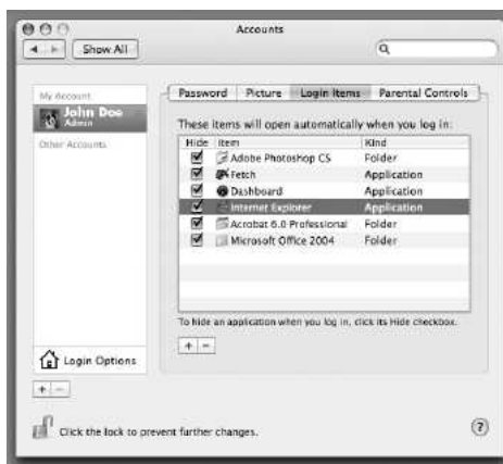
Clicking the minus sign under 'Login Items' is a remedy for a slow computer.
